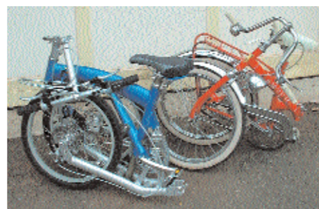
BELOW: The folding sequence is fine once you get the hang of it, and at 12kg, the bike isn't excessively heavy. The large main frame tube makes a convenient handle
