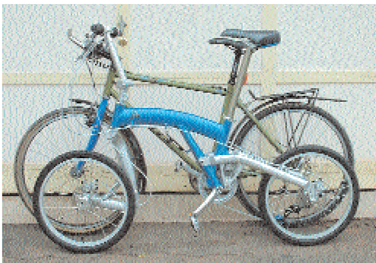
ABOVE AND RIGHT: Just as the manufacturers claim, the GoBike is pretty much identical to full-size bike geometry when it comes to wheelbase and seat and stem locations. It's noticeably longer in the wheelbase than many folders, helping the handling.
